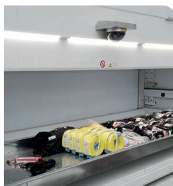
External bay lighting
